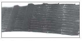
Cause of Failure — Web fabric wear caused by improper belt and pulley fit.
