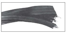
**Cause of Failure** — Worn sheave grooves allow the joined belt to ride too low cutting through to the top band. **Correction** — Replace sheaves and maintain proper belt tension and sheave alignment.
