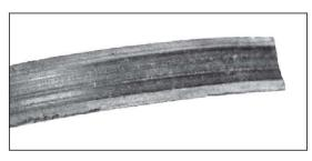
Cause of Failure — Back of the belt has been rubbing on a belt guard or other appurtenance.
