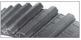
**Cause of Failure** — Fabric wear caused by insufficient belt tension or pulleys which are not to the standard PD pulley dimensions and tolerances.
